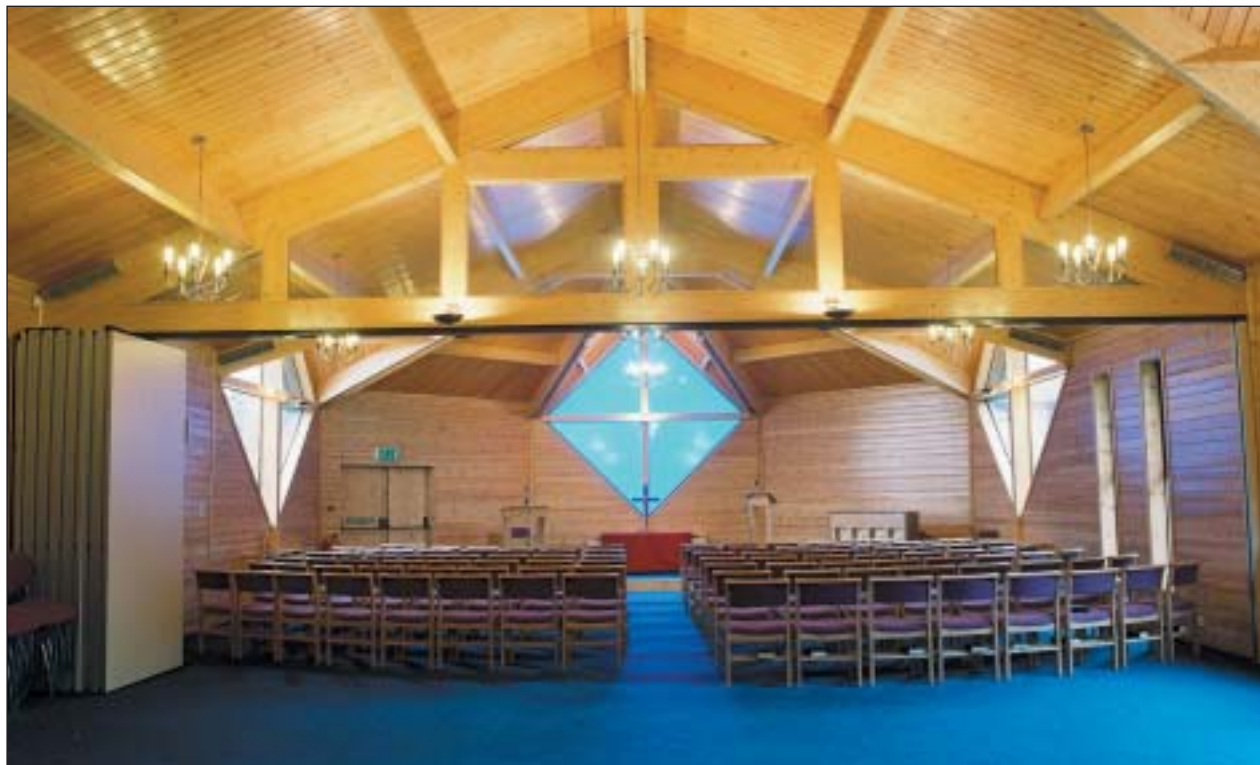
Sliding acoustic wall across the church
